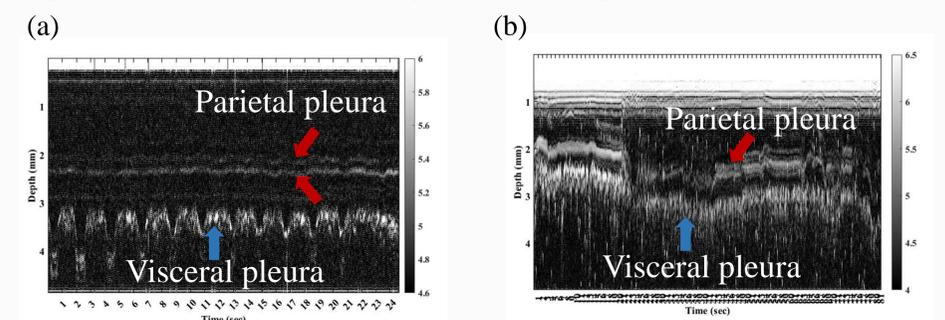
**Figure 3.** The ultrasound M-mode images of different materials-based ultrasound needle transducers in porcine in vivo experiment. (a) PMN-PT/ epoxy 1-3 composite, (b) PMN-PT.
