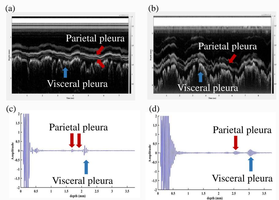
**Figure 2.** The ultrasound M-mode images and RF-mode of different materials-based ultrasound needle transducers in porcine lung in vitro experiment. (a, c) PMN-PT/ epoxy 1-3 composite, (b, d) PMN-PT.
