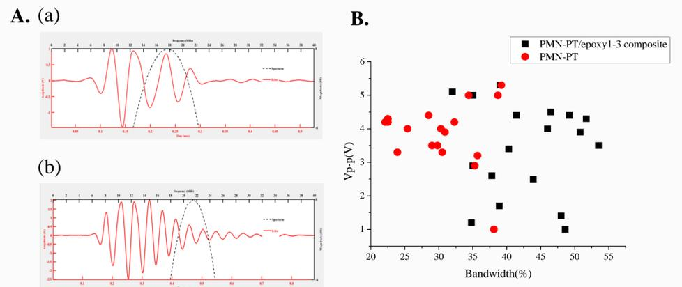
**Fig. 1.** A. Pulse-echo measurements and respective frequency spectra of different materials-based ultrasound needle transducers. (a) PMN-PT/ epoxy 1-3 composite, (b) PMN-PT. B. Amplitude and Bandwidth Scatter plot of PMN-PT/ epoxy 1-3 Composite and PMN-PT transducers.
