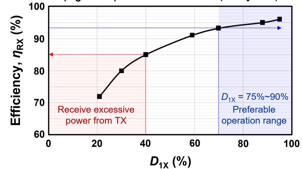
$\Box D_{1X}$  implies  $\eta_{RX}$ . Transmitter can perceive the load condition and further adjust the transmission power by utilizing duty ratio detector.
