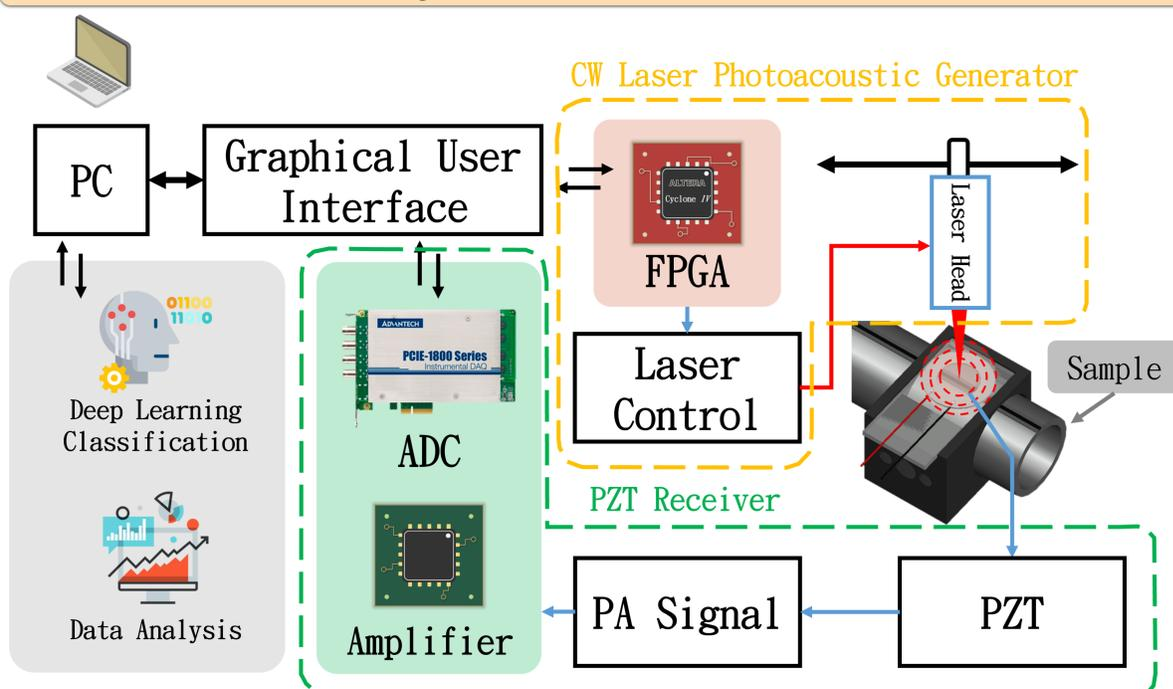
Figure 1. Architecture of the photoacoustic sensing system.
